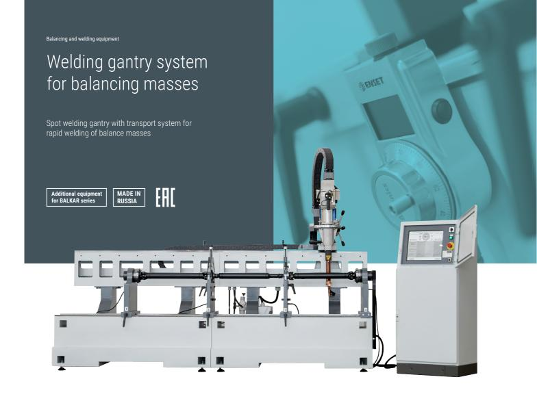
Spot welding gantry with a transport system for rapid welding of balance masses is an optional supplement to the BALKAR series machines. The gantry is used for automation of final correction of rotor unbalance by welding balancing masses. It is equipped with a high quality welding unit manufactured by TECNA, Italy. The operating algorithms are optimised to run the gantry and the balancing machine as a single unit.
